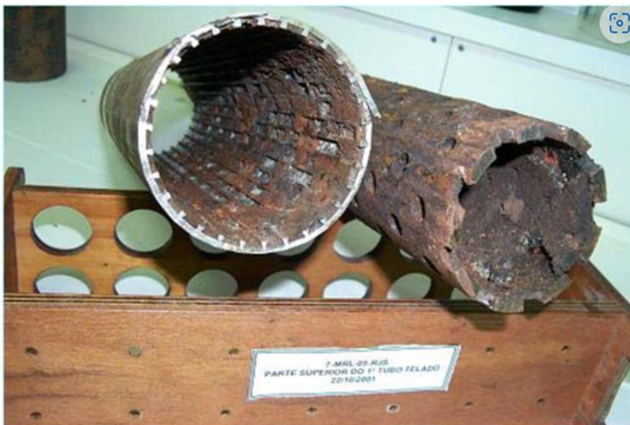
Figure 2 – Barium and strontium sulphate scale on sand screens.
